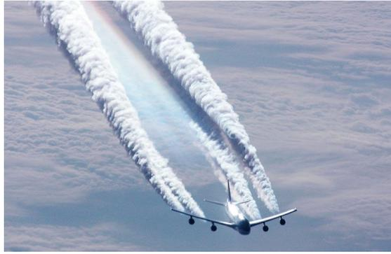
Figure 1: Wake of an airplane visualized by condensation behind the engines. The vorticity sheet is generated at the trailing edge of the wings.
