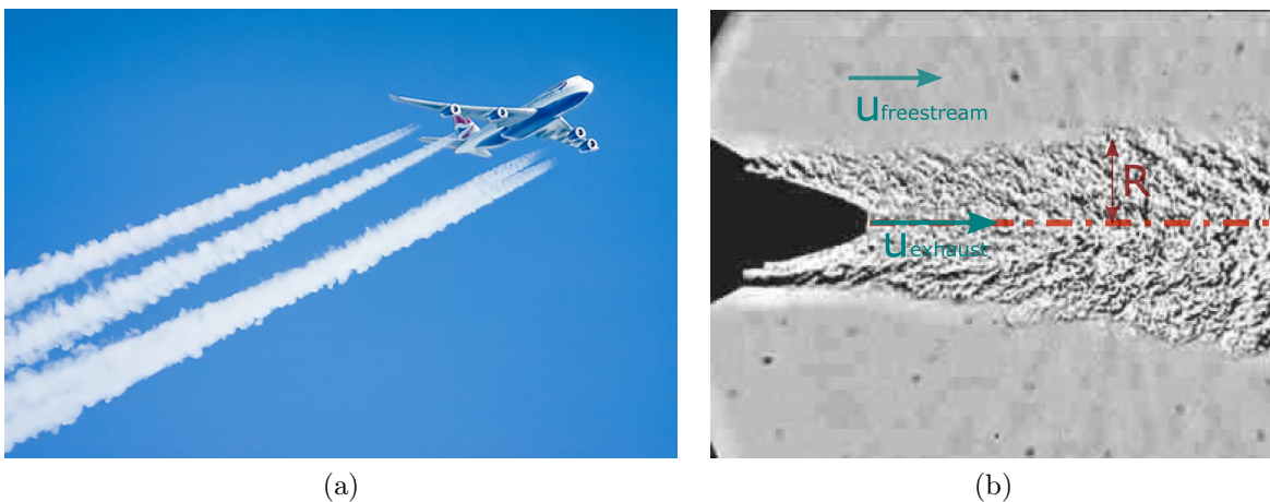
Figure 1: (a) Jet contrails in the wake of a Boeing 747 (source: www.wired.com/2009/05/climate-contrail-connection-contested ) (b) Schlieren image of the jet exhaust from a single engine (source: supersonic.eng.uci.edu/meaf/jse_round_m09u410.htm )
