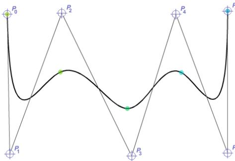
Figure 1: NURBS curve with cubic B-splines as basis functions. Source: [geometrie.foretnik.net](http://geometrie.foretnik.net).
