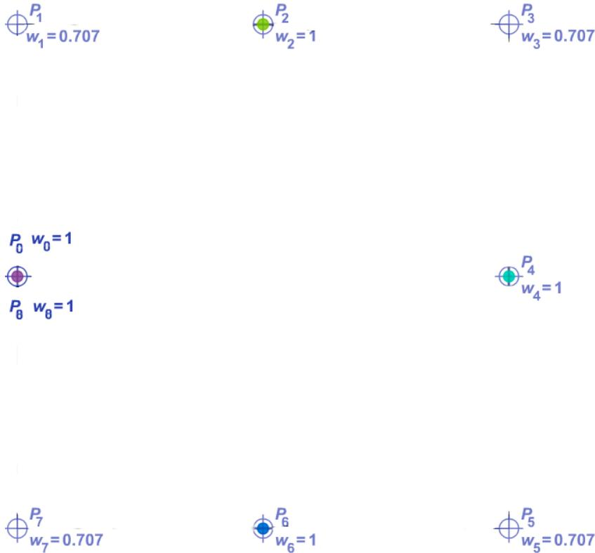
Figure 2: Locations of the control points and weights for the “hidden” spline. Source: [geometrie.foretnik.net](http://geometrie.foretnik.net).
