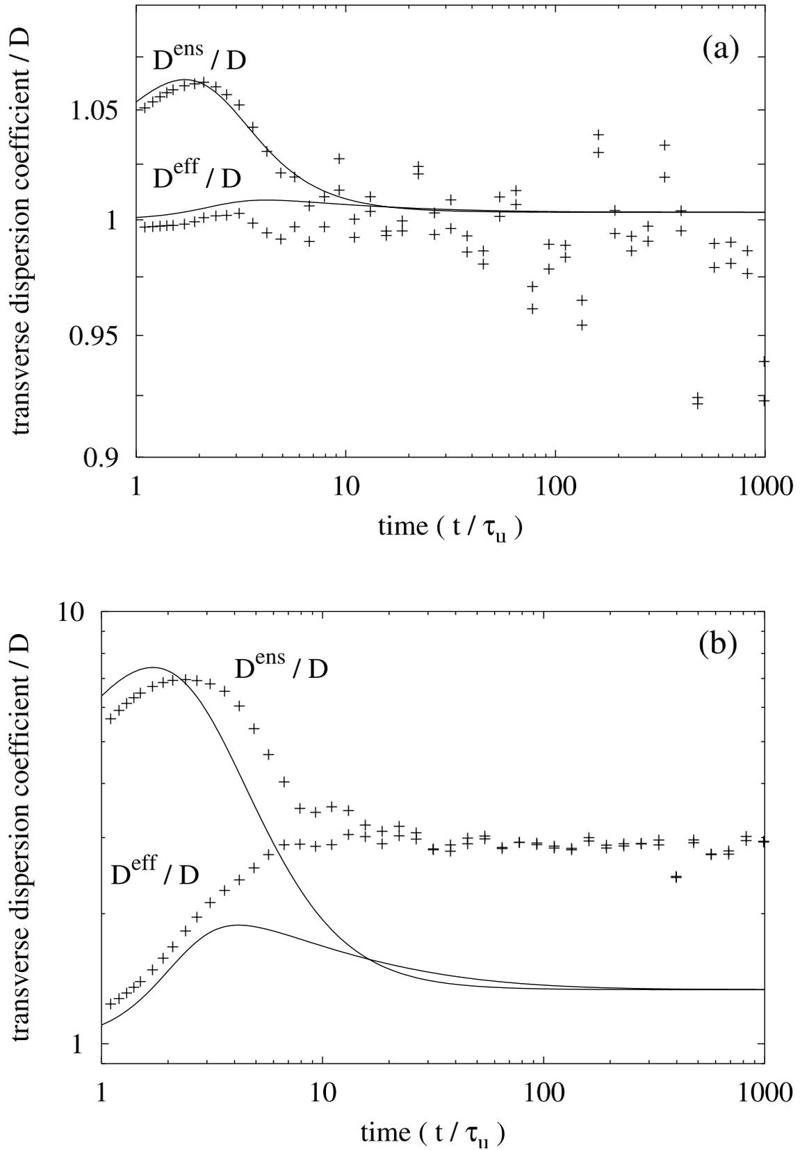
**Figure 5.** Temporal behavior of the transverse ensemble and effective dispersion coefficients normalized by  $D$  for  $\epsilon = \tau_u / \tau_D = 0.01$ , and the corresponding second-order expressions in  $d = 3$  (with (a)  $\sigma^2 = 0.01$  and (b)  $\sigma^2 = 1$ ,  $\bar{u} = 1$  m/d,  $l = 1$  m).
