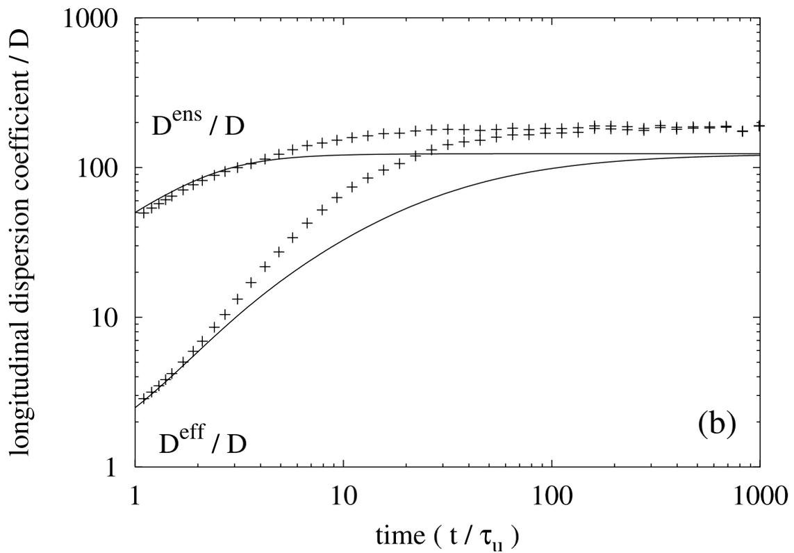
**Figure 4.** Temporal behavior of the longitudinal ensemble and effective dispersion coefficients normalized by  $D$  for  $\epsilon = \tau_u / \tau_D = 0.01$ , and the corresponding second-order expressions in  $d = 3$  (with (a)  $\sigma^2 = 0.01$  and (b)  $\sigma^2 = 1$ ,  $\bar{u} = 1$  m/d and  $l = 1$  m).
