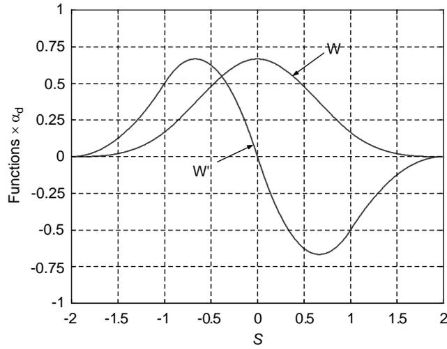
Fig. 3. Cubic spline kernel and its first derivative.
