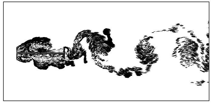
Figure 4: Instantaneous particle velocity at the position of the particles in the vicinity of the First Tacoma Narrows bridge (Larsen and Walther 1996).
