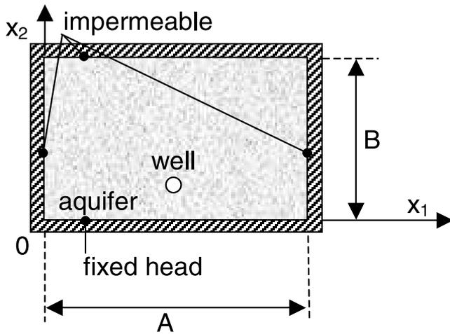
**Figure 2.** Aquifer domain of rectangular test cases with uniform recharge rate and constant pumping rate.
