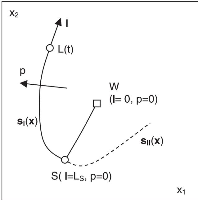
**Figure 1.** Locally orthogonal coordinate system with longitudinal ( $l$ ) and perpendicular ( $p$ ) coordinates of mean particle trajectory for catchment boundary, starting at well  $W$ , and passing by the stagnation point  $S$ .
