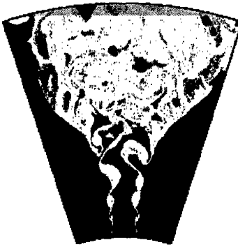
Figure 5: Controlled flow - Bifurcating Jet
