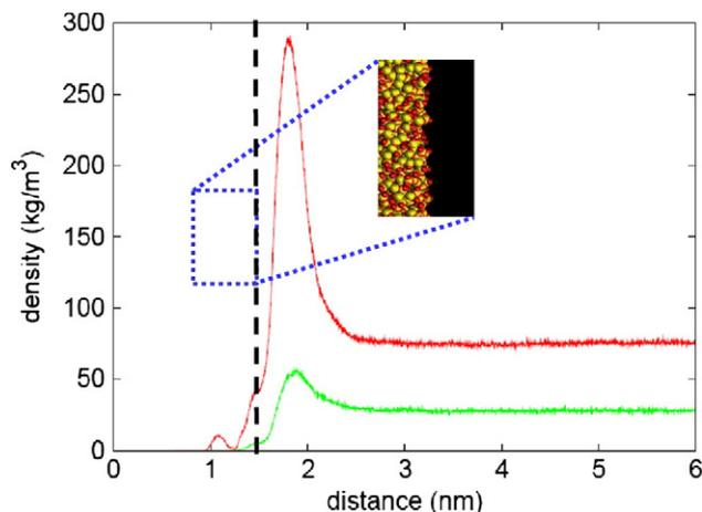
**Fig. 3.** Density profile of air at a silica surface at 300 K and 100 bar. The red line shows the  $N_2$  density profile; and the green line the  $O_2$  density profile. In this plot, the silica surface atoms are placed at ca. 1.5 nm.
