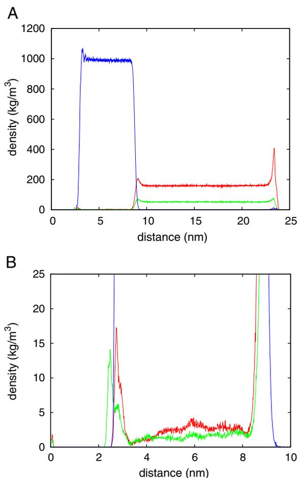
**Fig. 6.** Water slab on a silica substrate surrounded by air. Density profiles of water and air at 300 K and 200 bar. (A) Density profiles for the bulk zone of the system. (B) Details of the density profiles of air dissolved inside the water slab. The red line is the N<sub>2</sub> density, the green line is the O<sub>2</sub> density, and the blue line is the water density. The silica surface is located at ca. 2.7 nm, and it includes geometrical heterogeneities (molecular roughness).
