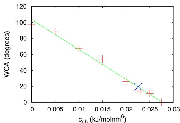
**Fig. 2.** Water contact angle (WCA) of a water nanodroplet on a silica surface as a function of the Buckingham interaction parameter  $C_{ab}$ . Red (+): WCA determined in vacuum; blue (x): the value fitted to the experimental WCA; green (–) linear fit to the computed data.
