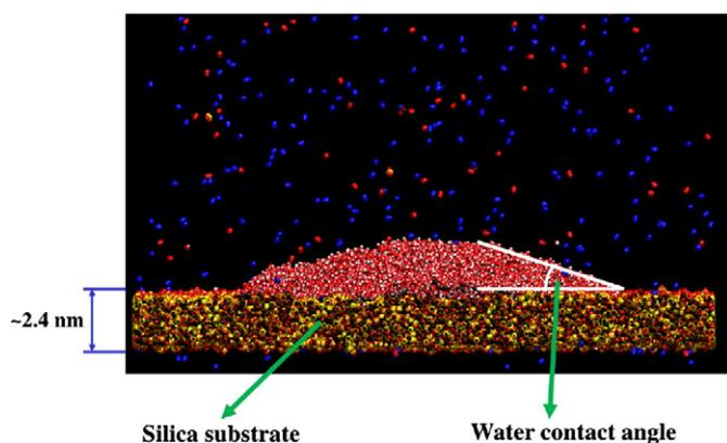
**Fig. 1.** Contact angle of a water nanodroplet on an amorphous silica slab. Snapshot from a MD simulation of a water nano-droplet mounted on a silica slab subject to a high air pressure (10 bar).
