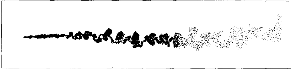
Fig. 4. Position of the vortices for the flow past a flat plate at Reynolds number 10^4 undergoing a harmonic pitch motion. The wake extends approximately 32 chord lengths downstream (not shown). v_r = 12 and t = 32 .
