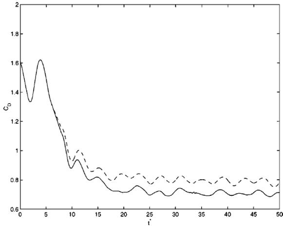
Fig. 6 Resulting drag coefficient for best populations, using all actuators (—) and only 4 most significant actuators (clustering technique, etc.)
