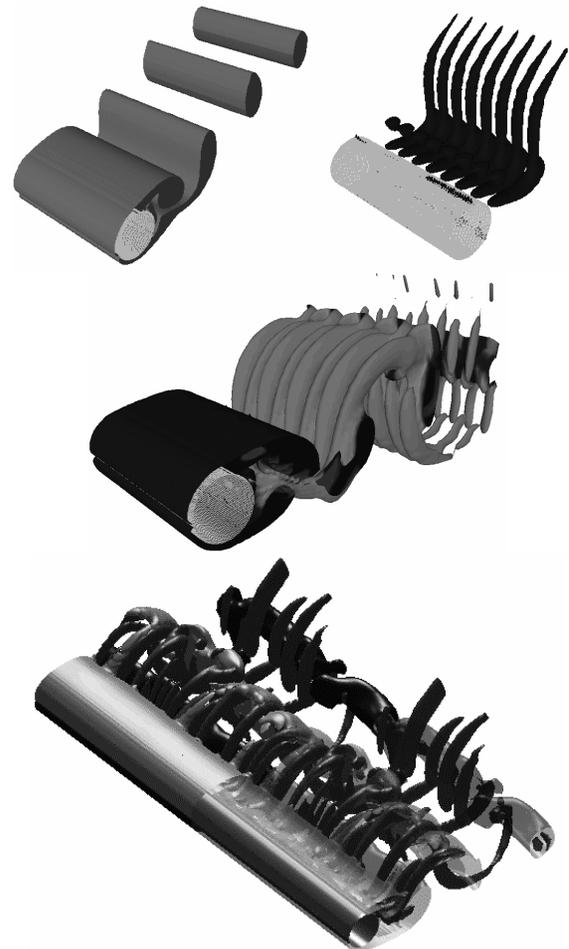
Fig. 1 Dynamics of cylinder wake in 3-D at  $Re = 300$ : 2-D wake (top left), first signature of instability (top right), resultant 3-D wake before saturation (middle), and post-transient established 3-D flow with fully developed hydrodynamic instabilities (bottom, from Poncet, 2004)
