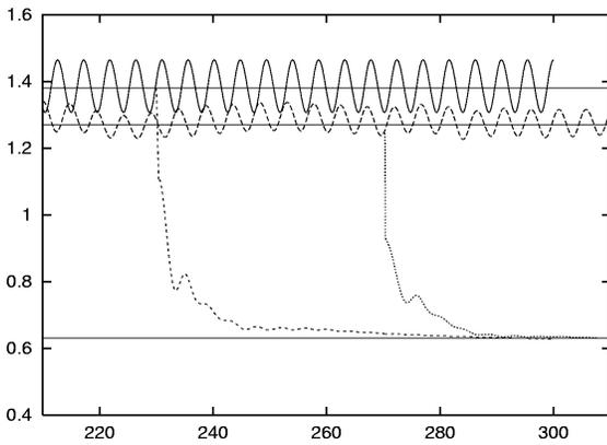
Fig. 10 Drag reduction and drag oscillation cancellation for 2-D flows (— uncontrolled, - - - controlled, activation at  $t = 230$ ) and 3-D flows (- - uncontrolled, ··· controlled, activated at  $t = 270$ )
