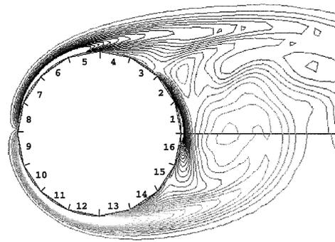
Fig. 4 Panel setup and flow example resulting from belt actuator configuration
