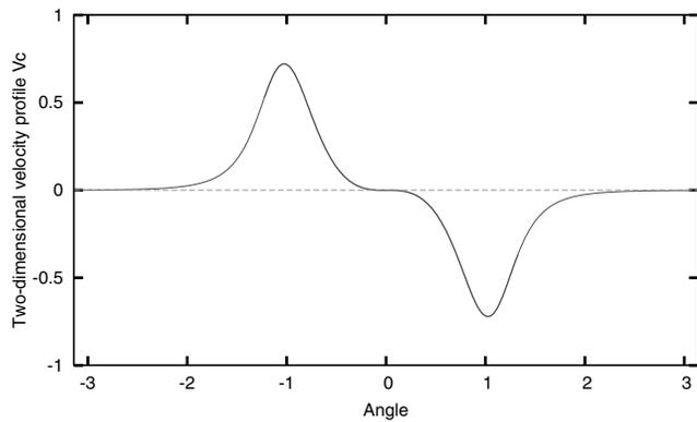
Fig. 7 Most probable velocity profile obtained with genetic algorithm (■) (top = absolute velocity with respect to segment number), and plot of fitting continuous smooth function  $f(\theta)$  from Eq. 7 (bottom, velocity versus angle)
