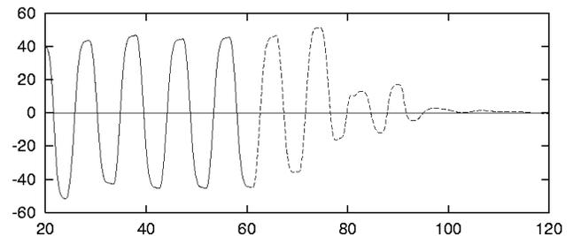
Fig. 9 Shedding (mean spanwise vorticity) before and after control activation (at  $t = 60$ ) for 2-D control of 3-D flow
