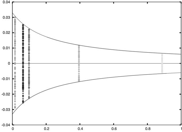
Fig. 15 Shedding reduction: drag coefficient (deviation from mean value) versus kinetic energy in low-energy control (small values of  $C$ ) and its fitting curve
