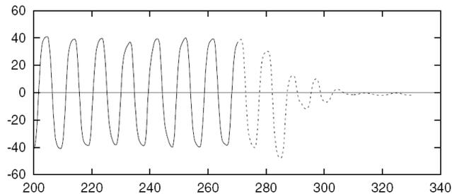
Fig. 11 Shedding (mean spanwise vorticity) before and after control activation (at  $t = 270$ ) for 3-D control of 3-D flow
