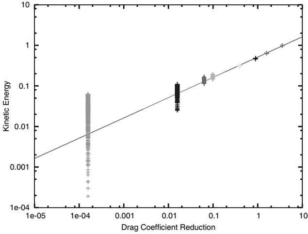
Fig. 14 Drag coefficient reduction versus kinetic energy in logarithmic scale, for various values of  $C$  (left to right: 0.01, 0.1, 0.2, 0.25, 0.5, 0.75, 1 and 1.5) and its square-root regression
