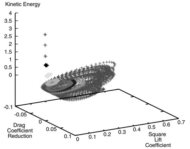
Fig. 17 Attractor: Drag coefficient/lift coefficient/energy (Eq. 11)
