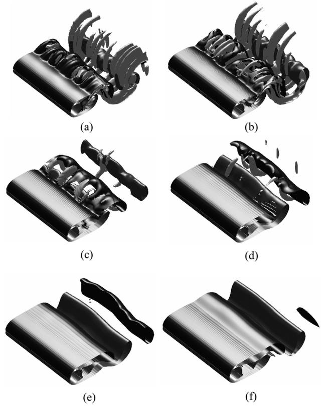
Fig. 8 Isovalues of vorticity after control activation with smooth velocity profile, at different times (a~f, respectively, at  $t = 270, 280, 290, 300, 310$  and  $320$ ), from Cottet and Poncet (2004)
