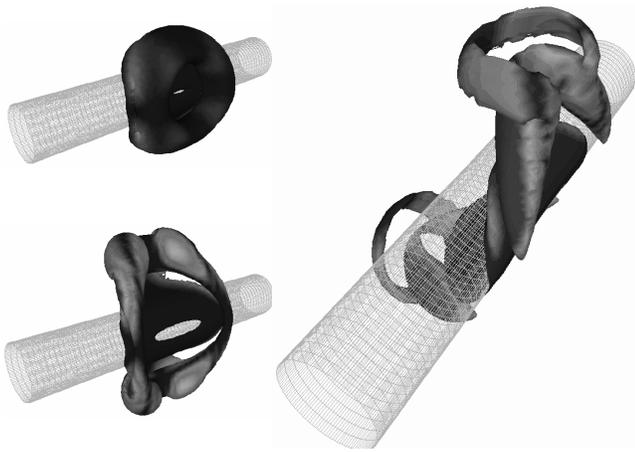
Fig. 2 Annular vortex and cylinder interaction, fusion between main ring and boundary layer, generating secondary ring-vortex (photos of vorticity at 3 different times)
