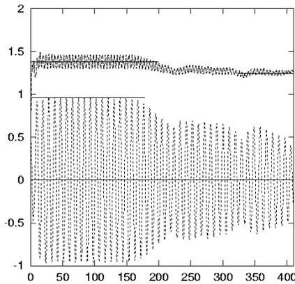
Fig. 3 Typical drag (—) and lift (---) coefficient of cylinder wake developing streamwise hydrodynamic instabilities at  $Re = 300$
