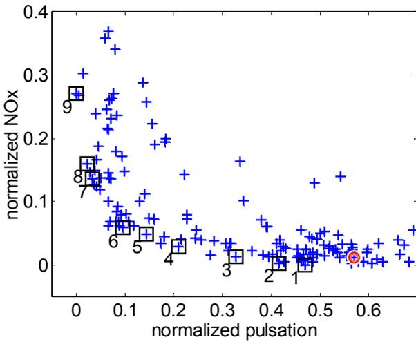
Figure 11. Optimization using digital valves. The numbered boxes correspond to the valve settings of figure 12.
