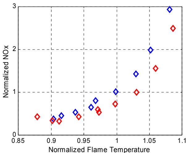
Figure 16. Combustion test at atmospheric conditions comparing the optimized burner against the baseline.
