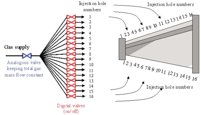
Figure 10. Schematic of the test rig using digital valves.
