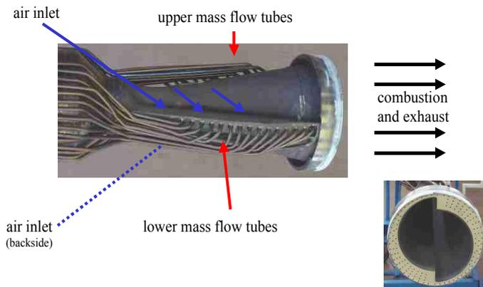
Figure 3. Sketch of the atmospheric combustion test-rig with a low-emission swirl stabilized burner. The fuel flow through the injection holes are the design variables of the setup. The  $\text{NO}_x$  emissions and the pulsation of the burner are the objectives to be minimized.
