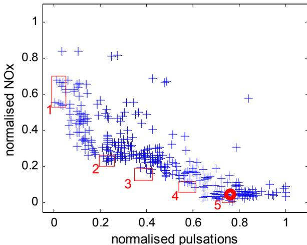
Figure 6. All measured solutions of the burner optimization run [plus symbol] and given standard burner configuration [circular symbol]. The 5 boxes mark the different areas along the nondominated front.
