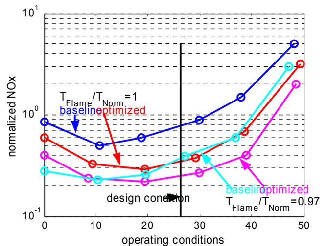
Figure 17. Combustion test at pressurized conditions comparing the optimized burner against the baseline.
