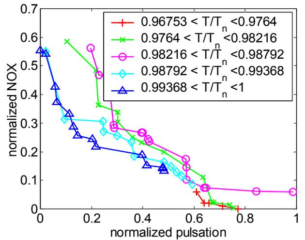
Figure 14. Pareto-optimal solutions (designs) dependent on flame temperature.
