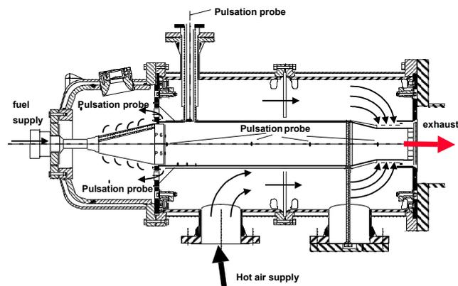
Figure 4. Schematic of the elevated pressure test facility
