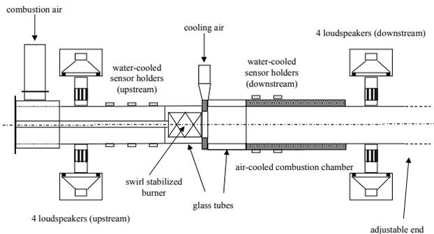
Figure 1. Schematic of the atmospheric test facility
