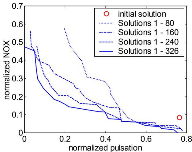
Figure 9. Convergence towards optimal design. Shown are the Pareto-optimal designs after 80, 160, 240 and 326 optimization loops. Convergence is not yet complete.
