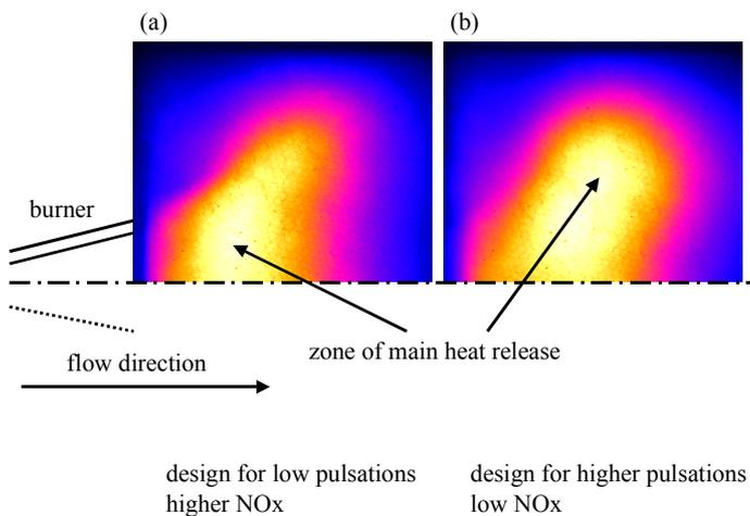
Figure 15. Flame visualization using OH chemiluminescence. Only the upper half of the symmetric flame is displayed. (a) flame shape for a low pulsation but higher  $\text{NO}_x$  design. (b) flame shape for low  $\text{NO}_x$  but higher pulsations.
