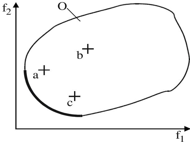
Figure 5. Illustration of the dominance principle a two-objective minimization problem. The solution  $a$  is dominating  $b$ , since  $a$  is superior in both objective values.  $a$  is indifferent to  $c$ , since each solution is superior in one objective. From the set of all feasible solutions  $O$  the set of Pareto solutions is marked by a bold line.
