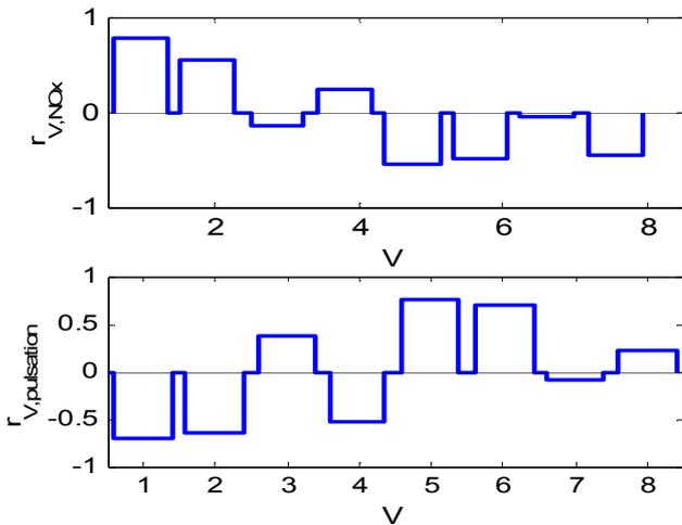
Figure 8. Correlation coefficient  $r$  between the mass flow through the valves  $V_{i,i=1,\dots,8}$  and the objectives  $NO_x$  and pulsation.
