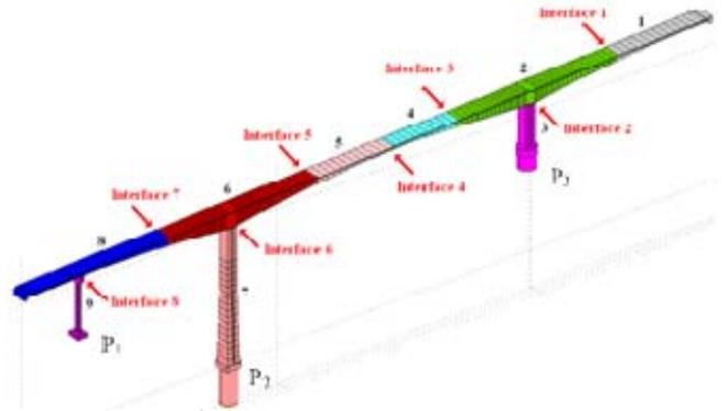
Figure 1. Components of FE model of bridge.
