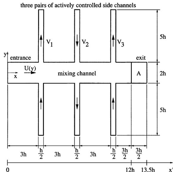
Fig. 2. Schematic of the flow configuration. Flow in the main channel is manipulated by controlling time-dependent flow from six secondary channels. The mixing rate is averaged in the region  $A$ .
