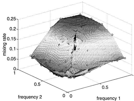
Fig. 4. Surface of the mixing rate as a function of the two actuation frequencies, constructed from points computed during the optimization (O).
