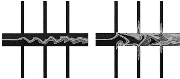
Fig. 3. Snapshots of the concentration field of the flow actuated by the frequencies in the three side-channel pairs  $\mathbf{x} = (1/2, 1/2, 1/2)$  (left) obtained by theoretical arguments, and by the optimal frequencies  $\mathbf{x} = (0.14, 0.32, 0.50)$  (right) obtained using evolutionary optimization.
