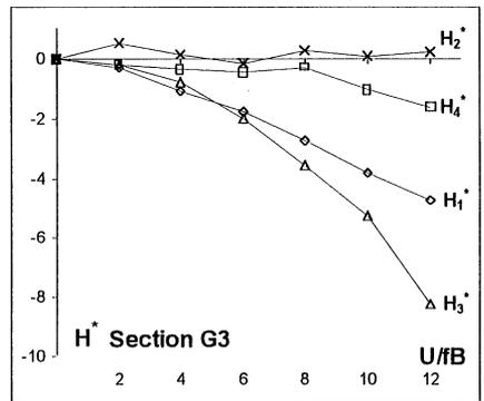
Fig. 5. Aerodynamic derivatives obtained from discrete vortex simulations of the flow about the generic sections G1, G2, G3, G4 and G5 in forced oscillatory motion.
