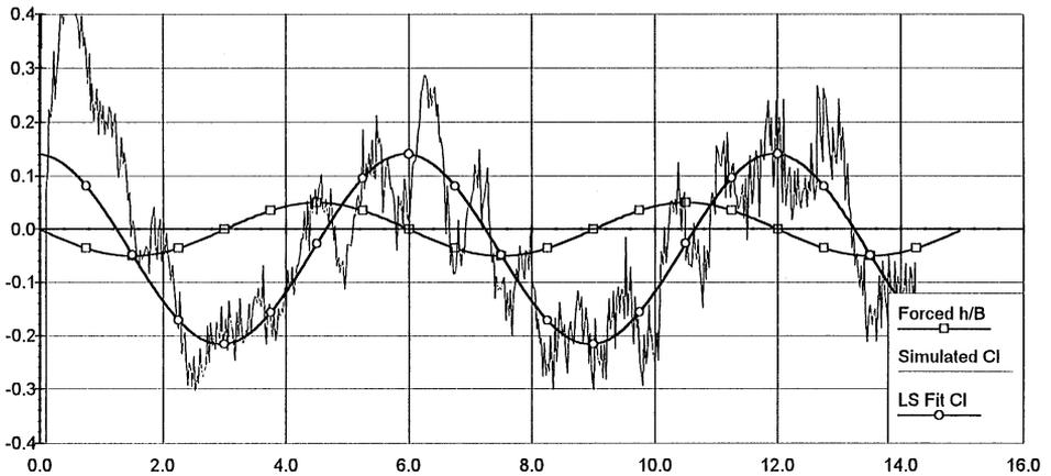
Fig. 4. Forced non-dimensional vertical bending  $h/B$ , simulated  $C_L$  time-trace and corresponding least-squares fit at  $U/fB = 6$  obtained for the G1 cross-section.
