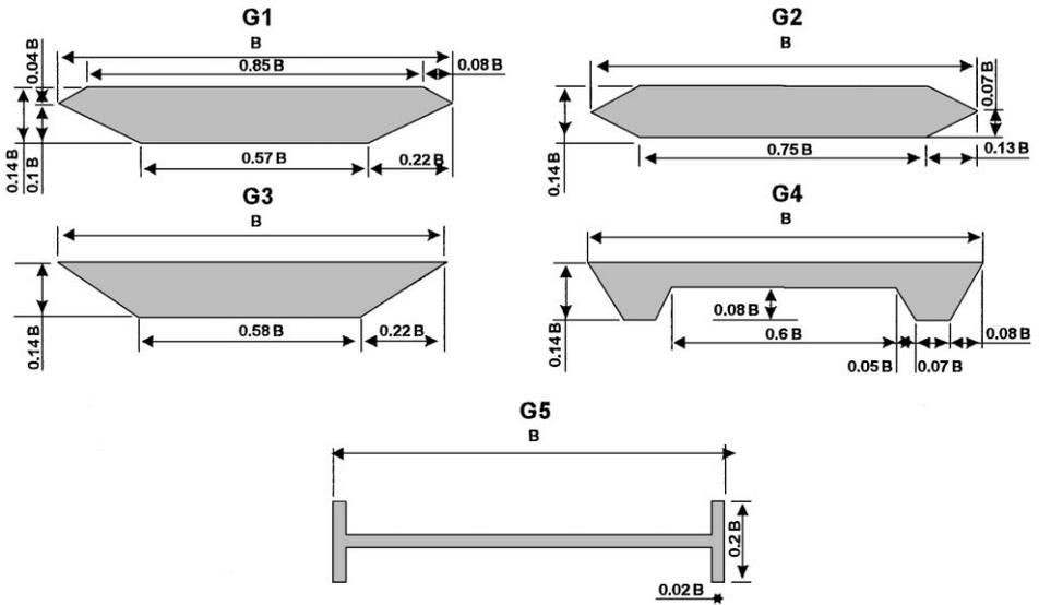
Fig. 1. Geometry of generic bridge girder cross-sections considered in the present study.
