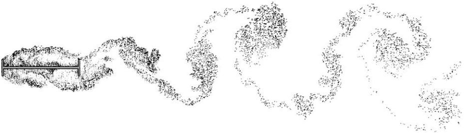
Fig. 3. Simulated von Kármán vortex street developing in the wake of section G5. Flow visualisation by plotting the positions of vortex particles at a given instant in time.
