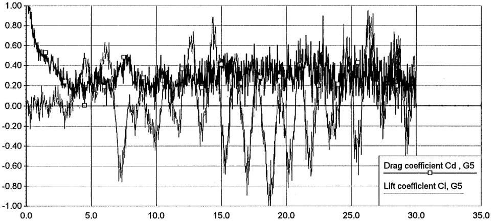
Fig. 2. Development of drag coefficient  $C_D$  and lift coefficient  $C_L$  for cross-section G5.
