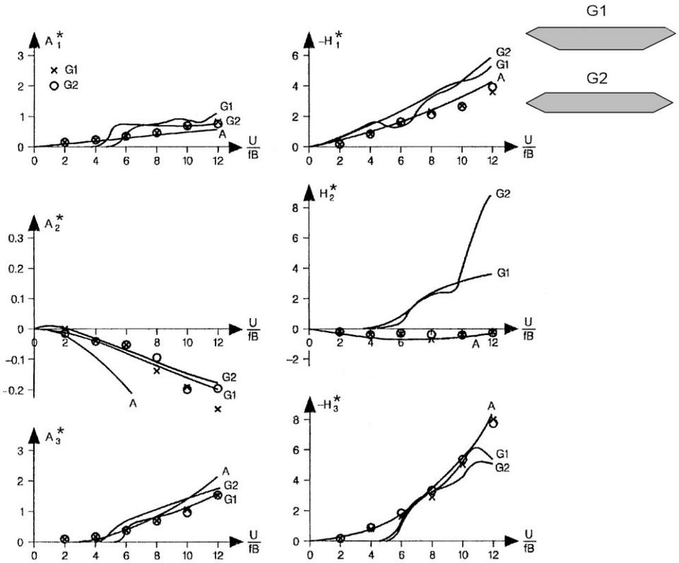
Fig. 6. Comparison of aerodynamic derivatives obtained from discrete vortex simulations to aerodynamic derivatives obtained from wind tunnel tests. Sections G1 and G2.
