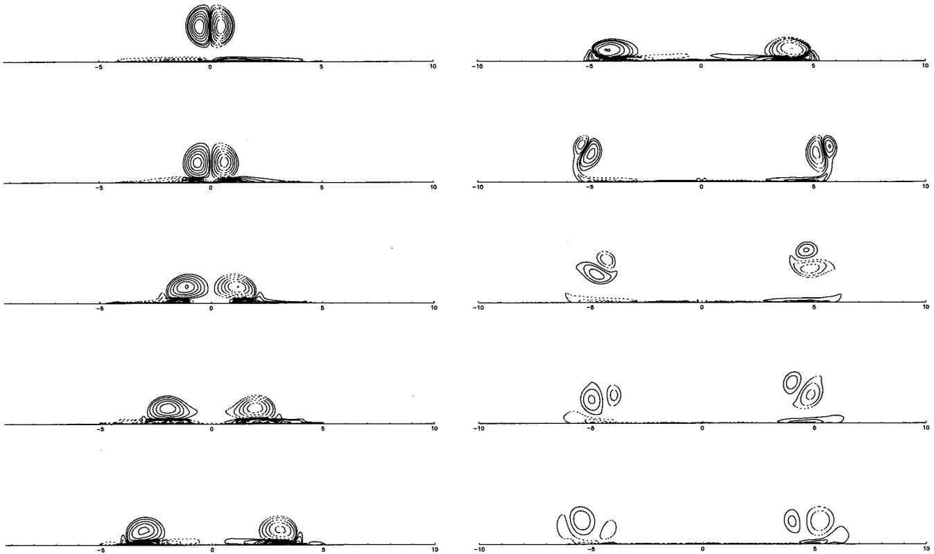
FIG. 9. Configuration 2b: *Controlled Wall-Vortex Interaction*. Contours at  $T=0.0, 0.2, 0.5, 1.0, 1.5, 2.0, 3.0, 4.0, 5.0, 6.0$  (top to bottom, left to right).
