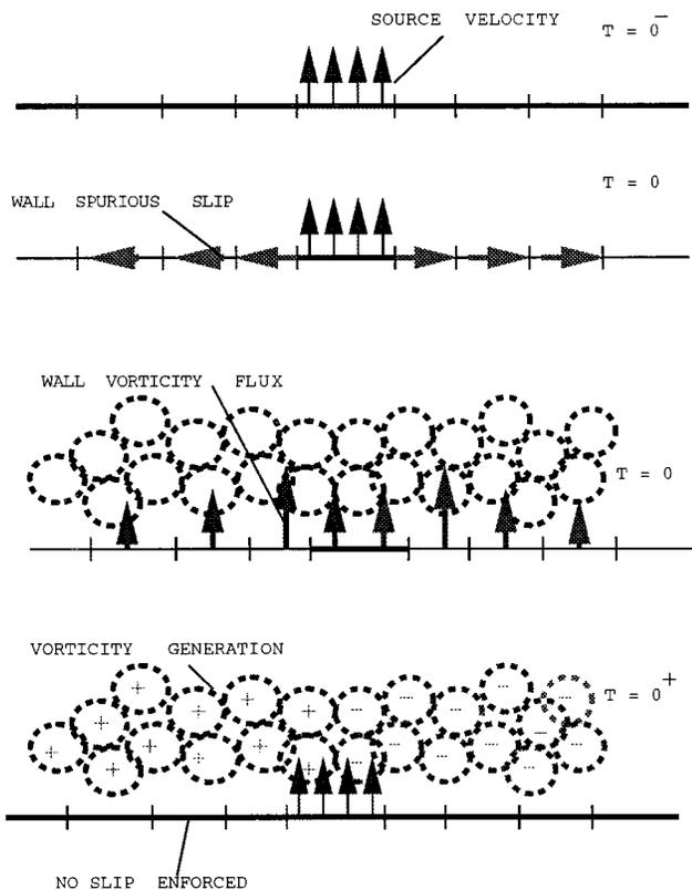
FIG. 2. Slip cancellation algorithm. The slip velocity and wall vorticity flux are averaged over wall segments.
