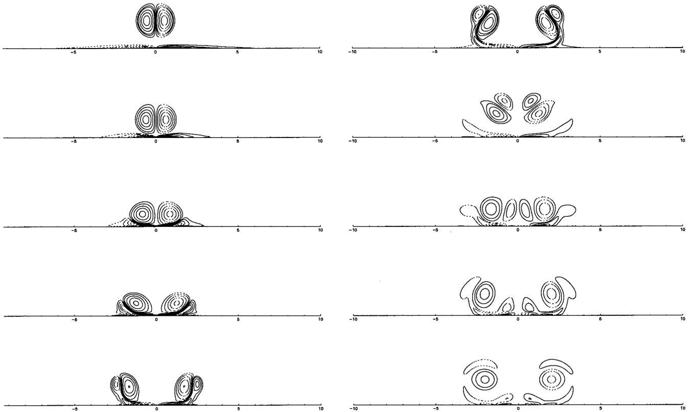
FIG. 3. *Uncontrolled* interactions of a vortex dipole with a wall. Contours at  $T=0.0, 0.2, 0.5, 1.0, 1.5, 2.0, 3.0, 4.0, 5.0, 6.0$  (top to bottom, left to right).
