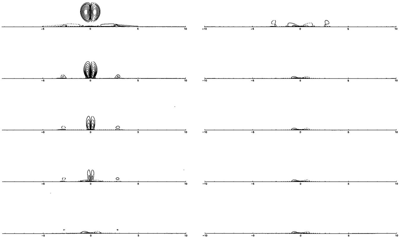
FIG. 5. Configuration 1b: *Controlled* wall–vortex interaction. Contours at  $T=0.0, 0.2, 0.5, 1.0, 1.5, 2.0, 3.0, 4.0, 5.0, 6.0$  (top to bottom, left to right).
