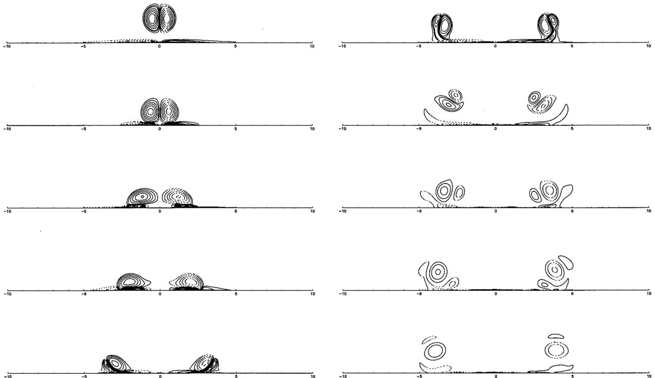
FIG. 8. Configuration 2a: *Controlled* wall–vortex interaction. Contours at  $T=0.0, 0.2, 0.5, 1.0, 1.5, 2.0, 3.0, 4.0, 5.0, 6.0$  (top to bottom, left to right).
