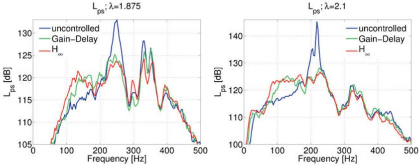
**Fig. 2** Comparison of the pressure spectra for the uncontrolled, Gain-Delay controlled and  $\mathcal{H}_\infty$  controlled plant. Both controllers are NH-CMA-ES optimized. Left:  $\lambda = 1.875$ , right:  $\lambda = 2.1$ .
