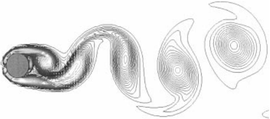
FIG. 8. Vorticity contours for a vortex wake at  $Re = 200$ .
