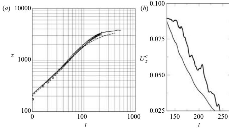
FIGURE 12. (a) Temporal evolution of the ring position, measured as the location of the maximum of  $|\omega|$ . Circles denote the experiment Weigand & Gharib (1994), the solid line corresponds to ring A (scaled), and the dashed line to ring B. (b)  $U_z^c$  of ring A (thin solid line), and  $\Gamma$  (bold solid line). The values of  $\Gamma$  have been scaled to allow a qualitative comparison of the decay.
