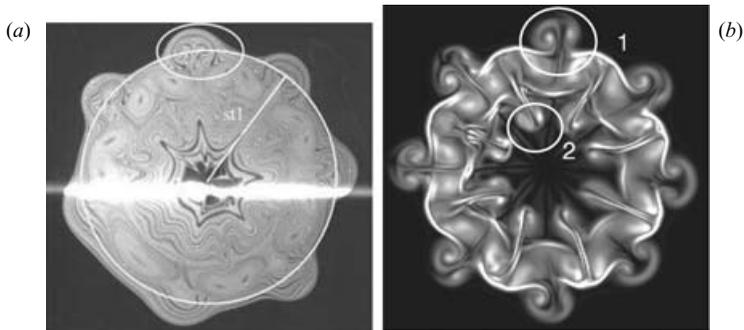
FIGURE 2. (a) Dye visualization of the secondary structures in the experiment (reproduced from Dazin *et al.* 2006b). (b) Vorticity magnitude in the present simulation (1: outer dipoles, 2: inner dipoles).
