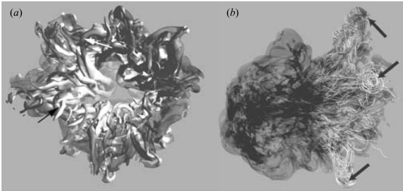
FIGURE 11. (a) Isosurface of  $|\omega| = 1.7$  for ring B at  $t = 108.29$  (viewed from behind). The surface is coloured by the strength of streamwise vorticity, where white regions denote high  $|\omega_z|$  and dark ones weak  $|\omega_z|$  respectively. Arrows denote hairpin vortices shed from the inside of the turbulent core. (b) Isosurface of  $|\omega| = 0.41$  for ring B at  $t = 120.53$ . Arrows denote the ring-like structures in the wake of the vortex.
