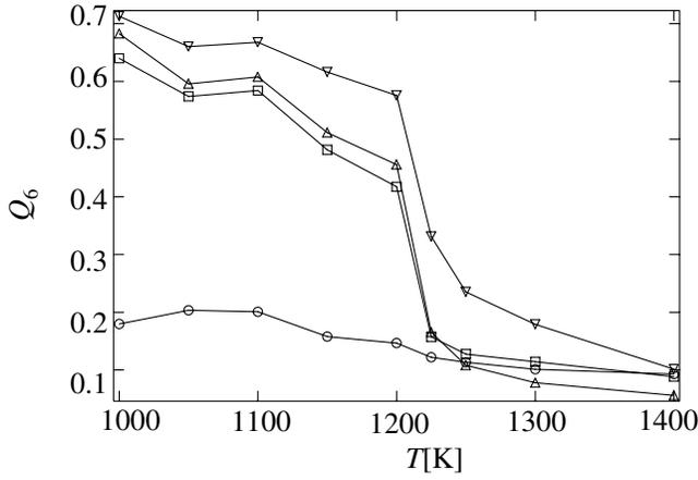
FIG. 3. Two-dimensional orientation order parameter  $Q_6$  at different temperatures: Case ( $N_{\text{Au}} = 1316$ ,  $n = 30$ ). Circles: first layer (innermost); squares: second layer; up triangles: third layer; down triangles: fourth layer (outermost).
