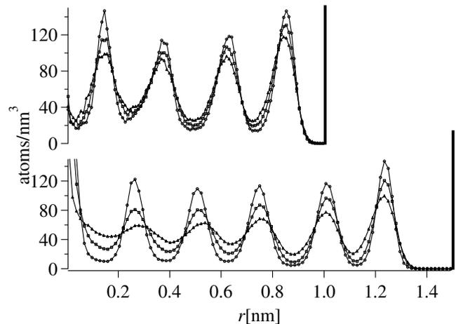
FIG. 2. Radial density profiles for the case at different temperatures. Circles,  $T = 1100$  K; squares,  $T = 1200$  K; triangles,  $T = 1400$  K. (a) The case ( $N_{\text{Au}} = 775$ ,  $n = 30$ ), with  $T_S = 1150$  K, and (b) the case ( $N_{\text{Au}} = 4983$ ,  $n = 40$ ), with  $T_S = 1215$  K.
