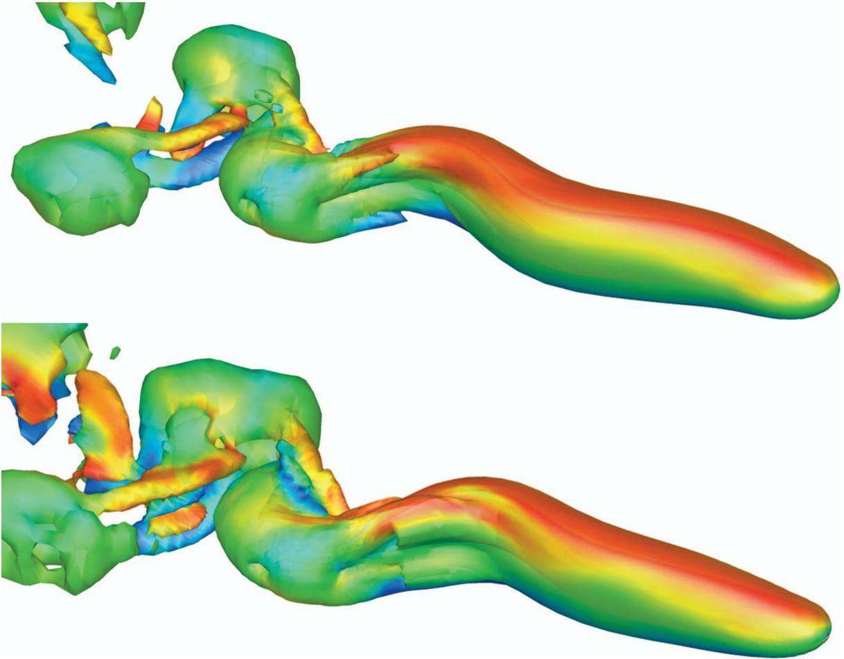
FIG. 1. (Color) Flow structure of the efficient (top) and fast (bottom) swimming motions visualized by plotting isosurfaces of vorticity magnitude  $\|\omega\| = 2$  colored by spanwise vorticity  $\omega_y$  (enhanced online).
